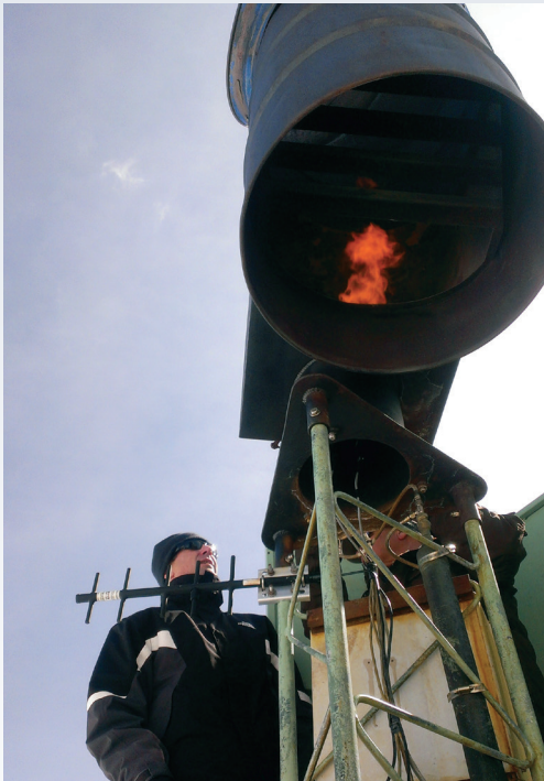
Aircraft or ground-based generators are used to burn a silver iodide solution to release microscopic silver-iodide particles that can assist in the formation of ice crystals in clouds.
