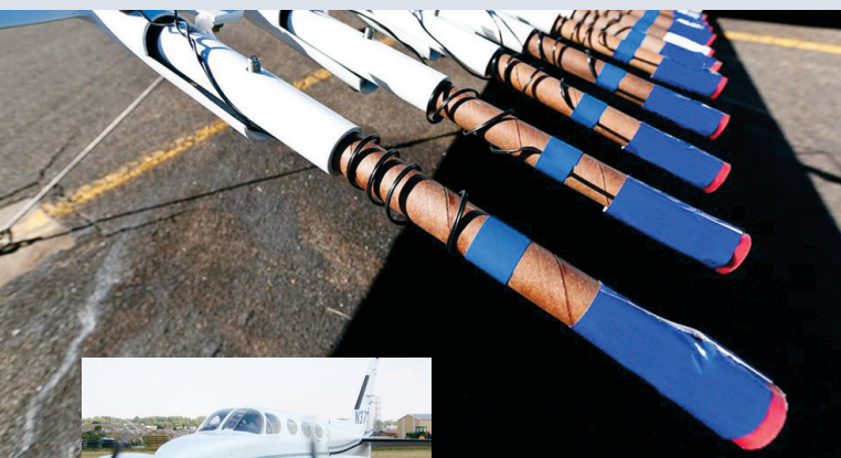
Burn-in-place flares are mounted on the aircraft wing to disperse silver iodide in a cloud.
