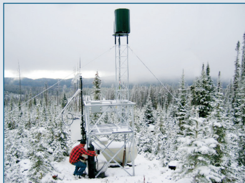
A ground-based generator is used to burn a silver iodide solution to release microscopic silver-iodide particles which can create additional ice crystals, then snow, in winter clouds. Research has shown that placing equipment at high elevations increases cloud seeding effectiveness.
